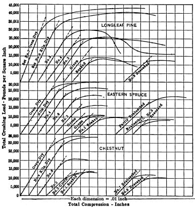
Fig. 14.—Relation between amount of compression and crushing load in pieces varying from an oven-dry to a soaked condition. (Compression parallel to grain—pieces  $1\frac{1}{2}$ "  $\times 1\frac{1}{2}$ "  $\times 5\frac{3}{4}$ ").
